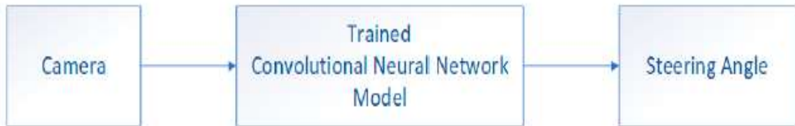
Figure . Block diagram of an end-to-end autonomous driving system.
